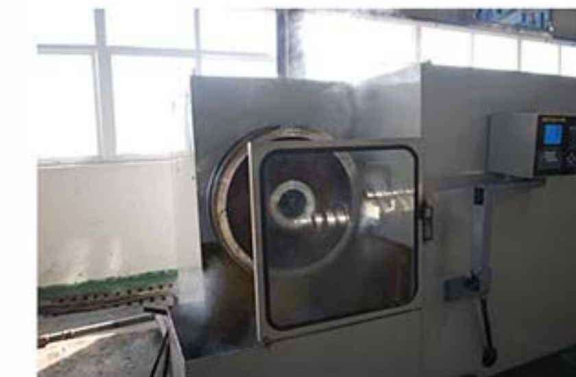
Medium -frequency quenching equipment
