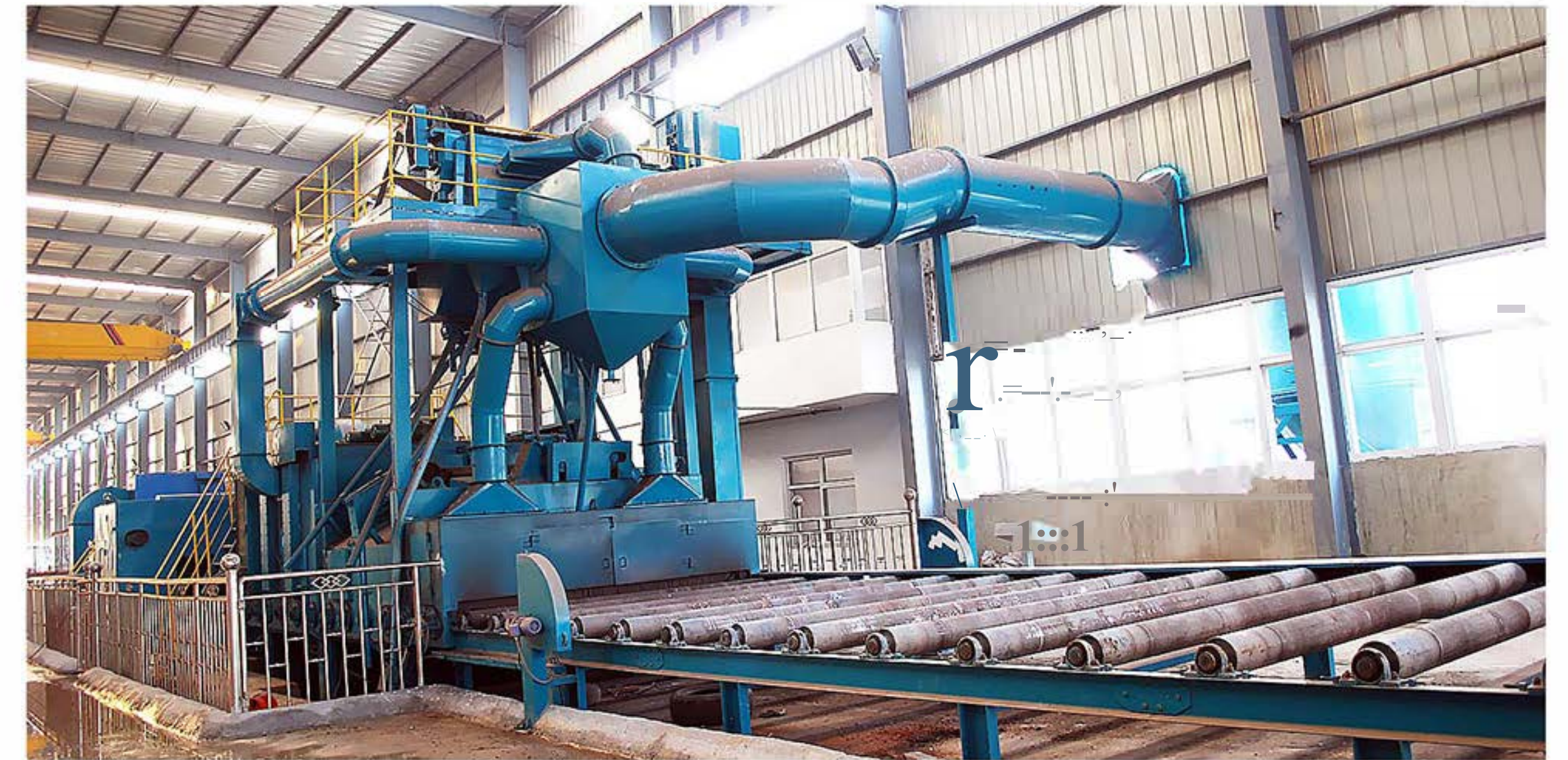
Large -size steel plate pretreatment shop-blasting machine
